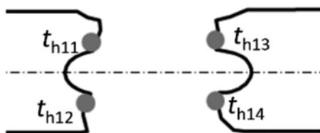
**Figure 9.5.3.** Schematic top view (left) and front view (right) of fracture surfaces of both specimen halves. Example locations for measurement of thicknesses  $t_{h11}$ ,  $t_{h12}$ ,  $t_{h13}$ , and  $t_{h14}$  on the specimen with a hole after the test
